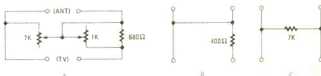
FIG. 5—GHOST ELIMINATOR is actually an L-pad attenuator as shown in a. Equivalent circuit when adjusted for minimum signal is shown in b. When adjusted for maximum signal, equivalent circuit is shown in c.
